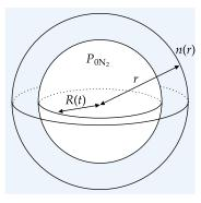
In spherical coordinates for a scalar field n(r) the gradient and Laplacian are written as such:
